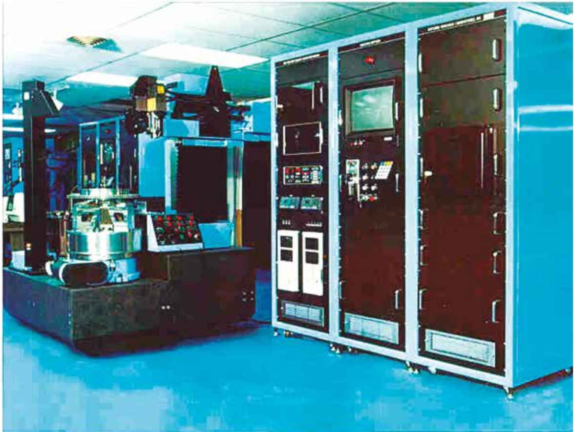
Figure 1. A Version 3 Retirement for Cause (RFC) Inspection Station
