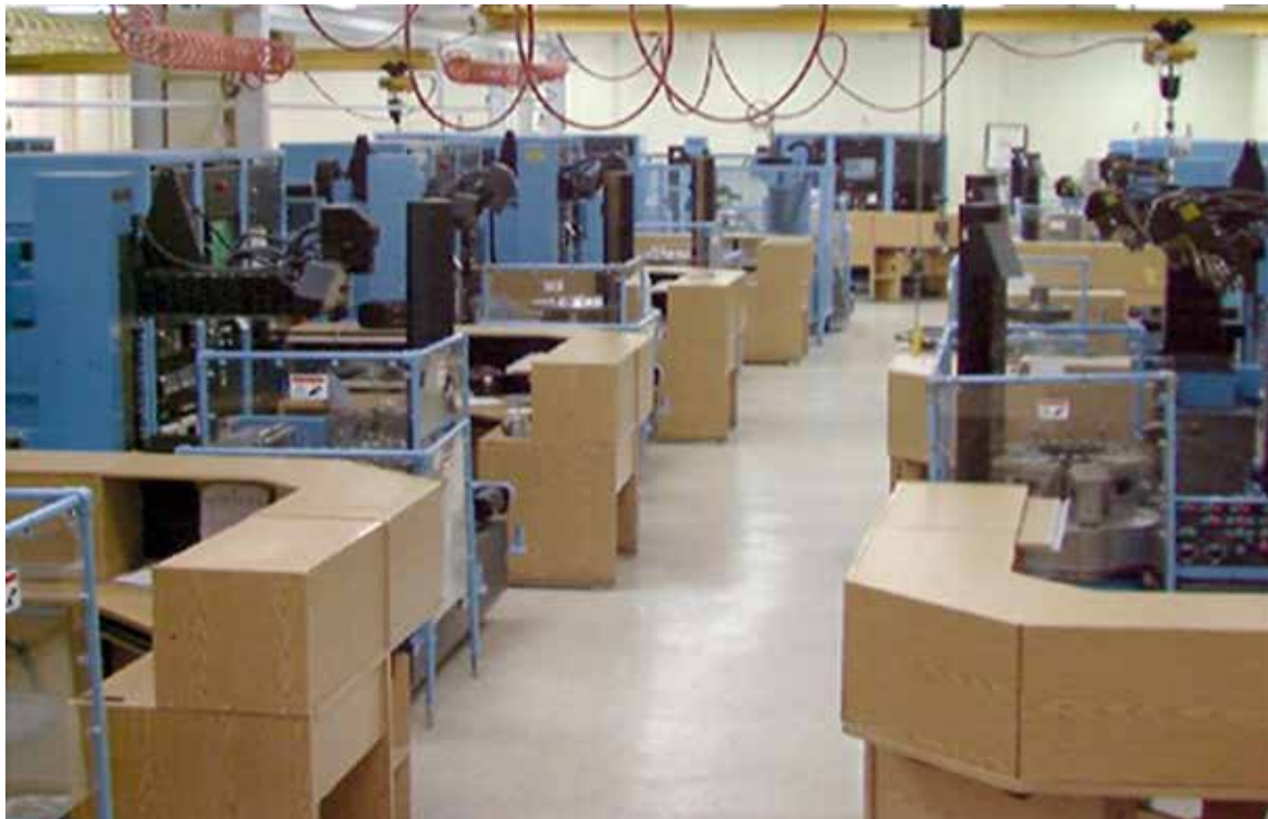
Figure 3. RFC inspection stations operating at an engine overhaul facility
