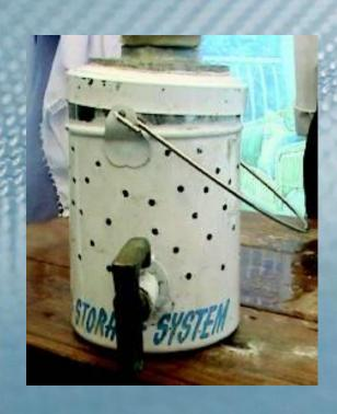
The rural refrigerator developed by two children works on the principle of evaporation. There is an outer steel jacket having pores in the upper half. There is a main storage compartment made of copper and another inner compartment which acts as a cooler. The exterior of the storage compartment and interior of the inner compartment are covered with cotton lining. The outermost jacket and innermost jacket are filled with water which takes away the heat from storage compartment.
